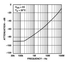
Figure 12. Off Isolation vs. Frequency
