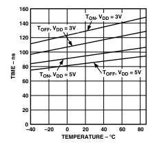
Figure 11.  $T_{ON}/T_{OFF}$  Times vs. Temperature
