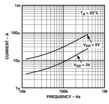
Figure 9. Input Current vs. Switching Frequency
