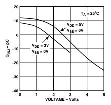
Figure 10. Charge Injection vs. Source Voltage
