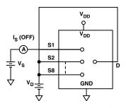
Test Circuit 2. I<sub>D</sub> (OFF)
