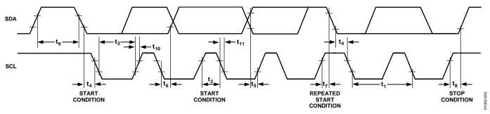
Figure 1. 2-Wire Serial Interface Timing Diagram
