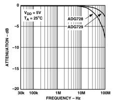
Figure 14. On Response vs. Frequency
