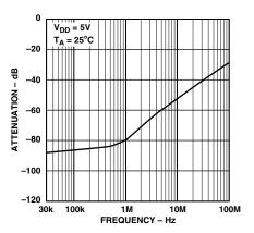
Figure 13. Crosstalk vs. Frequency
