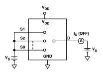
Test Circuit 3. I<sub>S</sub> (OFF)
