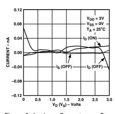
Figure 6. Leakage Currents as a Function of  $V_D$  ( $V_S$ )
