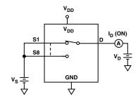
Test Circuit 4. I<sub>D</sub> (ON)
