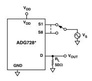
\*SIMILAR CONNECTION FOR ADG729 S1 IS SWITCHED OFF FOR OFF ISOLATION MEASUREMENTS AND ON FOR BANDWIDTH MEASUREMENTS OFF ISOLATION =  $20\text{LOG}_{10}(\text{V}_{\text{OUT}}/\text{V}_{\text{S}})$
