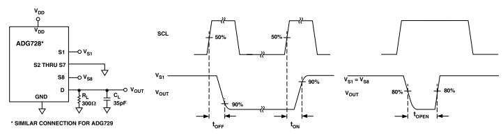
Test Circuit 5. Switching Times and Break-Before-Make Times
