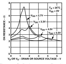
Figure 2. On Resistance as a Function of  $V_D$  ( $V_S$ ) for Single Supply
