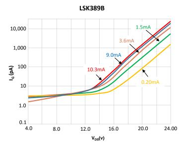
Figure 2. Gate Current (I<sub>G</sub>) vs. V<sub>DS</sub> vs. I<sub>D</sub>
