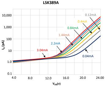
Figure 1. Gate Current ( $I_G$ ) vs.  $V_{DS}$  vs.  $I_D$
