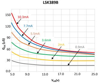
Figure 6. Output Conductance -  $G_{OS}$  vs.  $V_{DS}$  vs.  $I_{D}$
