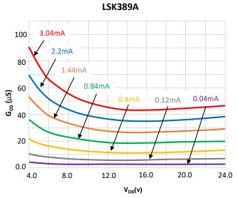
Figure 5. Output Conductance -  $\mathbf{G}_{\mathrm{OS}}$  vs.  $\mathbf{V}_{\mathrm{DS}}$  vs.  $\mathbf{I}_{\mathrm{D}}$
