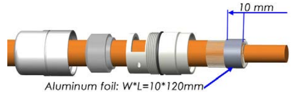
Step 4: Wrap foil over braided shielding
