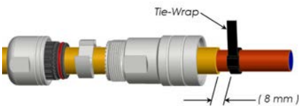
Step 3: Attach tie-wrap
