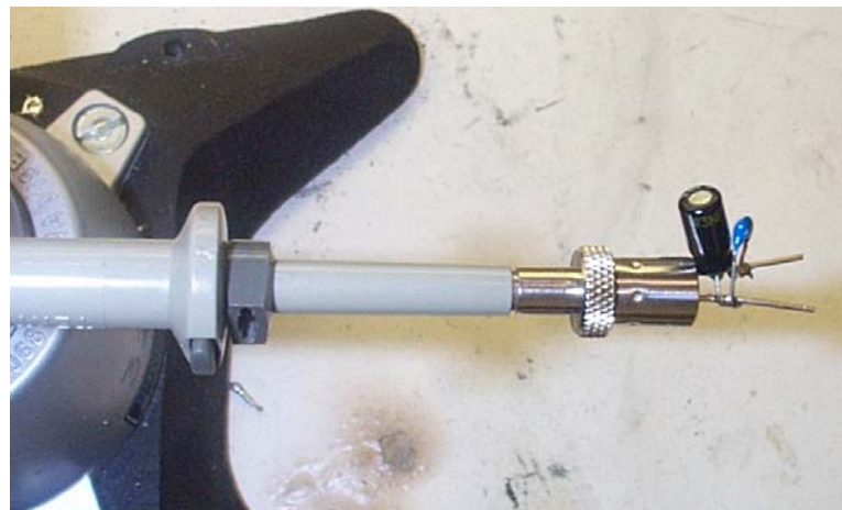
Figure 46 – Oscilloscope Probe with Probe Master 4987BA BNC Adapter (Modified with Wires for Probe Ground for Ripple measurement and Two Parallel Decoupling Capacitors Added).
