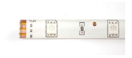
Cut away the waterproof overmolding at one end of the strip. The strips are symmetric so it doesn't matter which end you use.
