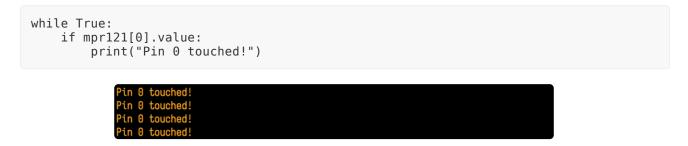
If you don't see any messages when you touch the inputs, you might need to ground yourself to the board by touching the GND pin on the board with one finger and then touching the input pads with another finger.
