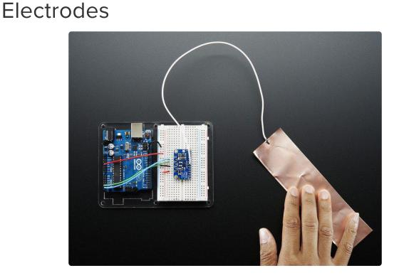
Once you have the MPR121 breakout working you'll want to construct electrodes. These are large conductive piece of copper, foil, paint, etc that will act as the "thing you touch"
