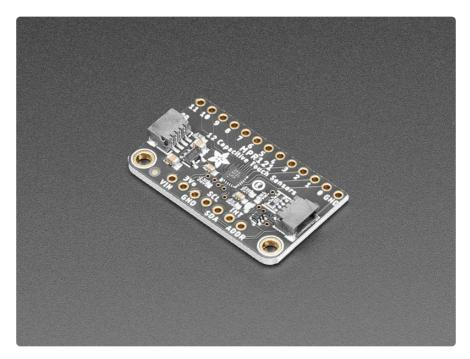
The MPR121 has support for only I2C, which can be implemented with nearly any microcontroller. You can select one of 4 addresses with the ADDR pin, for a total of 48 capacitive touch pads on one I2C 2-wire bus. Using this chip is a lot easier than doing the capacitive sensing with analog inputs: it handles all the filtering for you and can be configured for more/less sensitivity.
