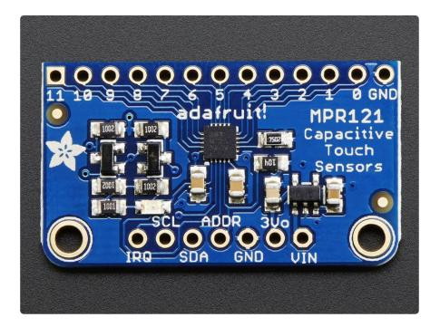
The pins are in a slightly different order on the original board from the STEMMA QT version. They function the same!
