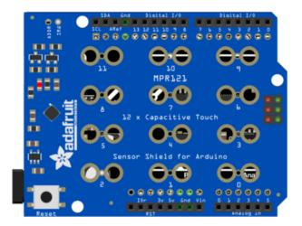
Solder the headers onto the shield, then simply connect it to your Metro M0.
