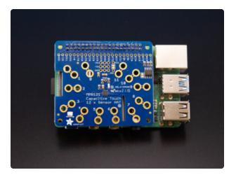
• Simply solder (https://adafru.it/drl) the header provided with the HAT onto the HAT, and attach the HAT to the Pi.
