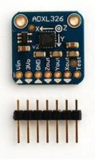
The ADXL326 can measure at least +/-16G(!) in the X, Y and Z axis. It is ideal for measuring more dynamic accelerations from high-performance land and air vehicles as well as for shock and impact measurements.
