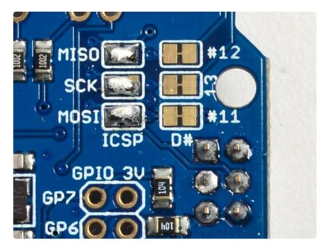
You can also cut the mini wire between the other three jumpers to 'release' the digital #11, 12 and 13 pins from being tied to the SPI pins. You can do this after you've gotten things working.
