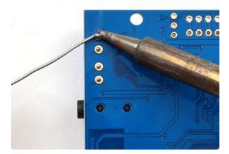
Solder the four pins with plenty of solder
