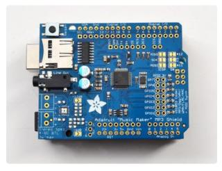
Place the shield on top so that all the little pins stick out through the matching holes in the shield. It should match up perfectly!
