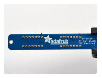
Turn over the PCB and bend oppositecorner pins of the modules out so that the modules are fixed in place against the PCB. Now is a good time to do a last check that you oriented the modules the right way!
