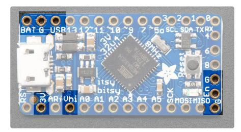
In addition to the three standard power pins, the 3V ItsyBitsy has a few more pins available for power sourcing:
