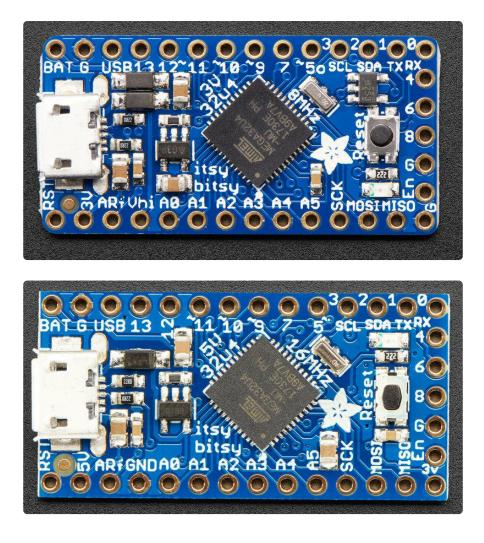
The pinouts for these are very similar except for the power pins which have different voltages!
