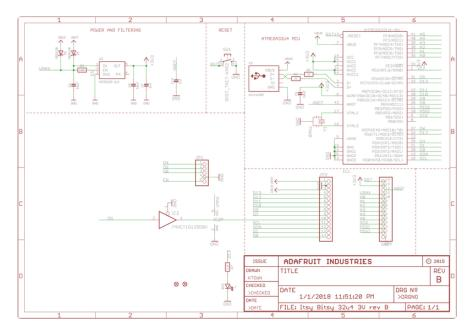
The 3.3V schematic regulator should be AP2112K-3.3
