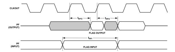
Figure 7. Programmable Flags Cycle Timing
