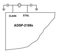
Figure 5. External Crystal Connections
