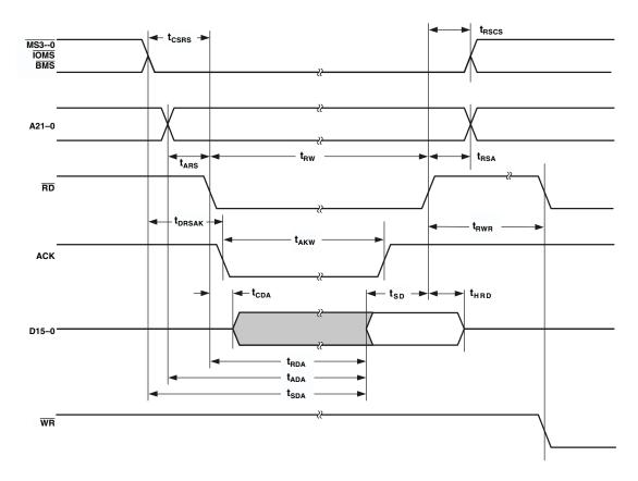
Figure 10. External Port Read Cycle Timing
