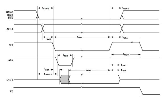
Figure 9. External Port Write Cycle Timing
