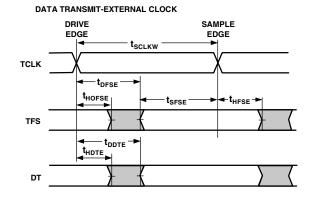
NOTE: EITHER THE RISING EDGE OR FALLING EDGE OF RCLK OR TCLK CAN BE USED AS THE ACTIVE SAMPLING EDGE.
