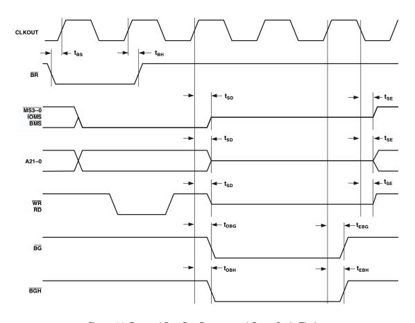
Figure 11. External Port Bus Request and Grant Cycle Timing
