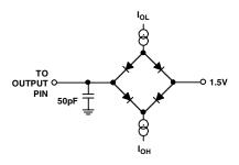
Figure 19. Equivalent Device Loading for AC Measurements (Includes All Fixtures)
