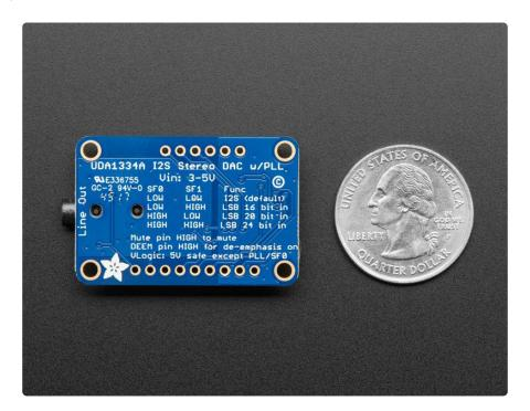
We put in plenty of ferrite beads, a low-dropout regulator, and the recommended band-pass filter so you get a very nice clean output. With a sine-wave generator we swept through 20-20KHz and saw no attenuation or distortion. Plug into either the 3.5mm stereo headphone jack or the breadboard-friendly pads. We think you'll be pleased with this DAC!
