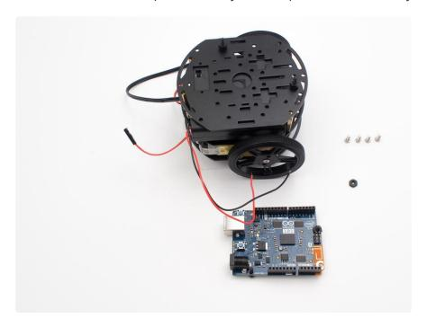
Screw the four brass standoffs into place with the small metal screws.
