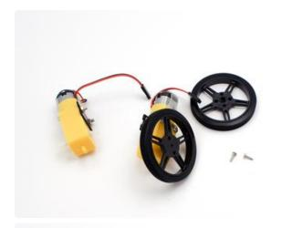
Fit the wheels onto the white knob on the motors, they will snap nicely onto the oval center.
