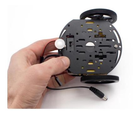
Place the battery box back in between the motors and stick it to the chassis
