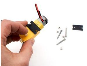
The metal panels go on the side with the red and black wires coming out.
