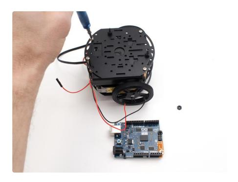
Place the Arduino 101 onto the top chassis layer, lining up the screws, then place the remaining nut onto the lower right screw to hold it in place. The upper left screw can't accommodate a nut due to the header row, but the screw will prevent the board from rotating.
