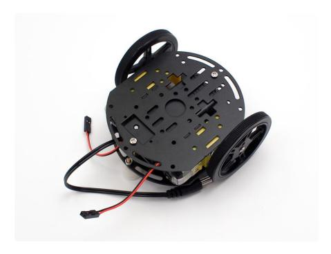
Place the middle chassis layer onto robot, making sure to fit the motor tabs into the slots of the layer, then screw in the two brass standoffs.
