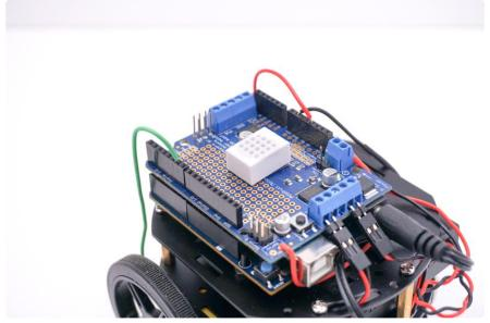
Open the Ada\_CurieBot\_RC\_NeoPixels sketch in the Arduino IDE and upload it to your robot.
