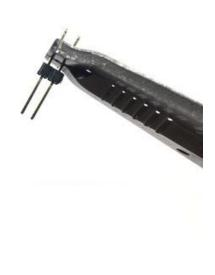
For this next step, you will need a set of pliers. First, grab the long header pins that are attached together and break them into 2 sets of 2 header pins. Then, grab them in the pliers like shown here, and then slightly bend them so they look like the next picture.
