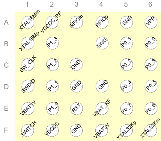
Figure 1: WLCSP34 ball assignment
