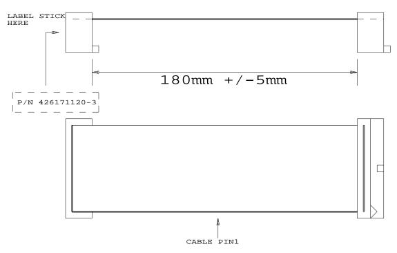
CONNECTOR: 25  $\times$  2 IDC CONNECTOR, 1.27  $\times$  2.54MM PITCH
