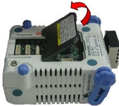
Figure 2-1. Acrylic Board Removal Method
