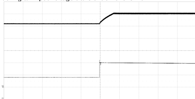
HRR product output at input voltage step 36-60 V, 10 ms/div Bottom trace – input voltage change 36-60 V, 20 V/div Top trace – resulting output voltage change, 2 V/div
