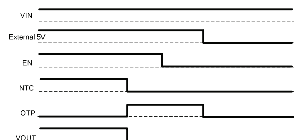
Figure 4: Normal Mode \rightarrow NTC protection Mode \rightarrow Transportation Mode
