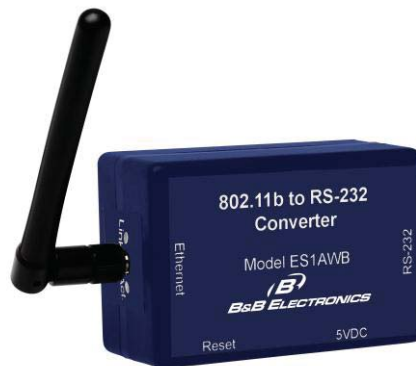
Figure 1. Front View of the ES1AWB Serial server
