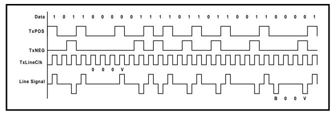
The user chooses between AMI or HDB3 line coding by writing to bit 4 of the I/O Control Register (Address = 0x01), as shown below.
