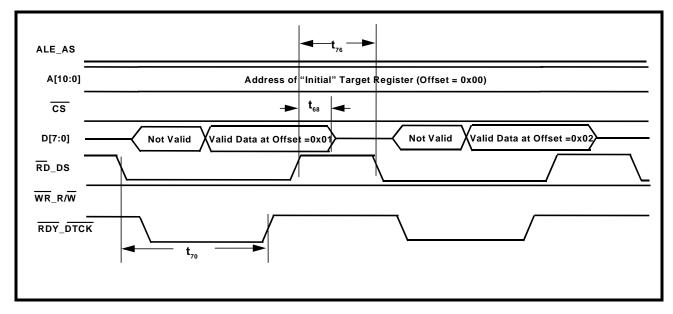
FIGURE 20. MICROPROCESSOR INTERFACE TIMING - INTEL TYPE WRITE BURST ACCESS OPERATION
