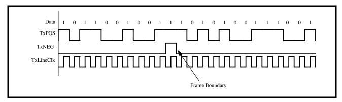
When the Transmit DS3 LIU Interface block is operating in the Bipolar (or Dual Rail) mode, then the contents of the DS3 Frame is output via both the TxPOS and TxNEG pins. If the Bipolar mode is chosen, then the DS3 data to the LIU can be transmitted via one of two different line codes: Alternate Mark Inversion
