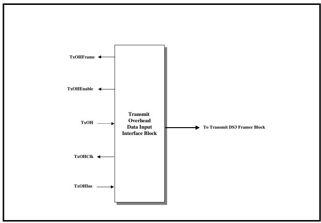
The E3, ITU-T G.751 Frame consists of 1536 bits. Of these bits, 1524 are payload bits and the remaining 12 are overhead bits. The XRT72L54 has been designed to handle and process both the payload type and overhead type bits for each E3 frame. Within the Transmit Section within the XRT72L54, the Transmit Payload Data Input Interface has been designed to handle the payload data. Likewise, the Transmit Overhead Input Interface has been designed to handle and process the overhead bits.
