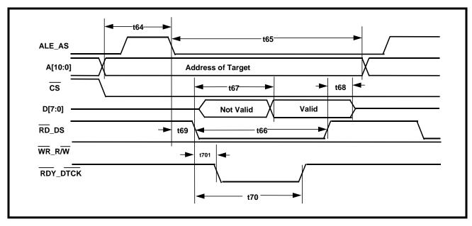
FIGURE 18. MICROPROCESSOR INTERFACE TIMING - INTEL TYPE PROGRAMMED I/O WRITE OPERATIONS
