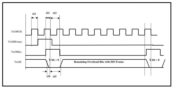
FIGURE 8. TIMING DIAGRAM FOR THE TRANSMIT OVERHEAD DATA INPUT INTERFACE (METHOD 2 ACCESS)
