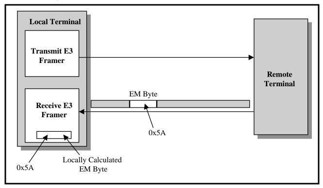
FIGURE 197. ILLUSTRATION OF THE LOCAL RECEIVE E3 FRAMER BLOCK, TRANSMITTING AN E3 FRAME (TO THE REMOTE TERMINAL) WITH THE FEBE BIT (WITHIN THE MA BYTE-FIELD) SET TO "0"
