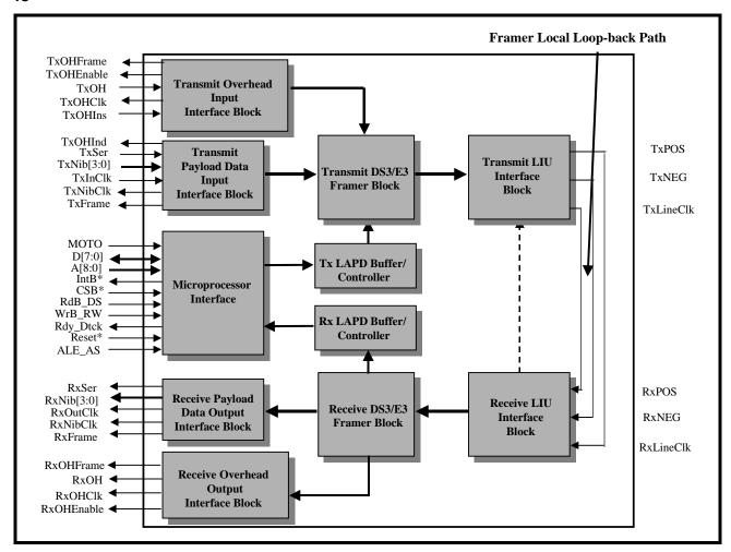
The user can configure the XRT72L54 into the Framer Local-Loop-back Mode by writing a "1" into bit-field
