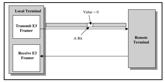
However, if the locally computed BIP-4 value does not match the BIP-4 value of the corresponding E3 frame, then the Receive E3 Framer block will do the following.
