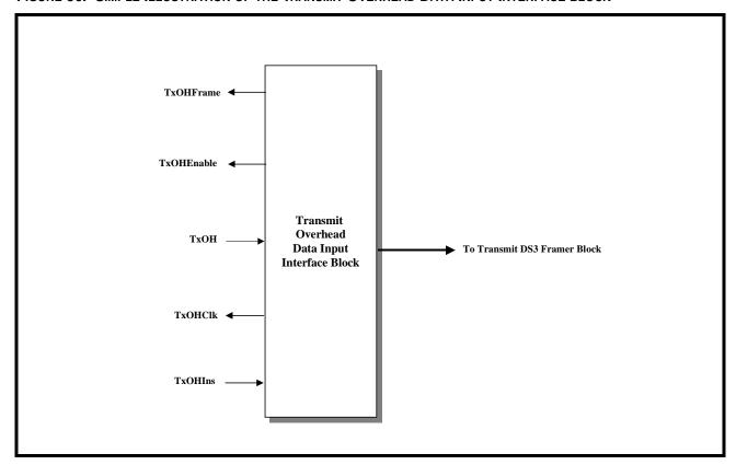
The DS3 Frame consists of 4760 bits. Of these bits, 4704 bits are payload bits and the remaining 56 bits are overhead bits. The XRT72L54 has been designed to handle and process both the payload type and overhead type bits for each DS3 frame. Within the Transmit Section within the XRT72L54, the Transmit Payload Data Input Interface has been designed to handle the payload data. Likewise, the Transmit Overhead Data Input Interface has been designed to handle and process the overhead bits.
