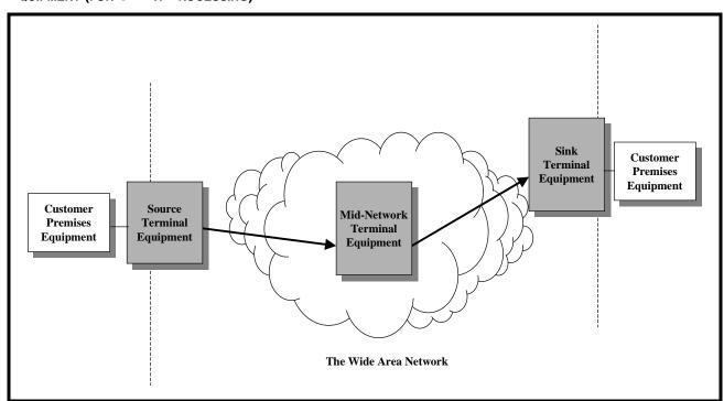
**Note:** The use of the terms Source and Sink Terminal Equipment are used to simplify this discussion of CP-Bit Processing. In reality, the Source Terminal Equipment (in Figure\_62) will also function as the Sink Terminal Equipment (for DS3 traffic traveling in the opposite direction). Likewise, the Sink Terminal Equipment (in Figure\_62) will also function as the Source Terminal Equipment.
