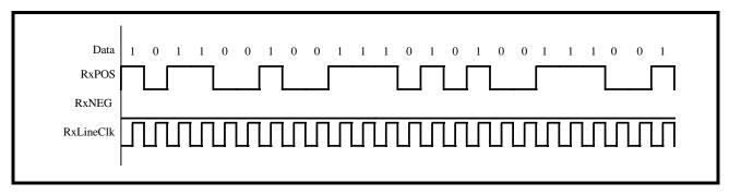
The user can configure the Receive E3 LIU Interface block to operate in either the Unipolar or the Bipolar
