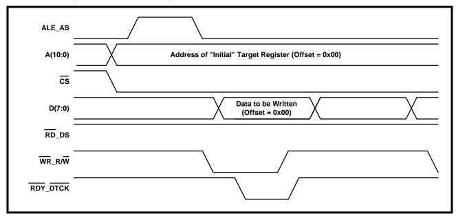
At the completion of this initial write cycle, the  $\mu C/\mu P$  has written a byte or word into the first register or buffer location (within the XRT72L54 DS3/E3 Framer) for this particular burst access operation. In order to illustrate this point, the byte (or word) of data, that is being written in Figure 31 has been labeled Data to be Written (Offset = 0x00).
