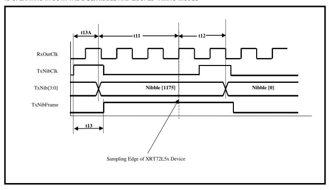
FIGURE 6. TIMING DIAGRAM FOR THE TRANSMIT PAYLOAD DATA INPUT INTERFACE, WHEN THE XRT72L54 DEVICE IS OPERATING IN THE DS3/NIBBLE AND LOCAL-TIMING MODES
