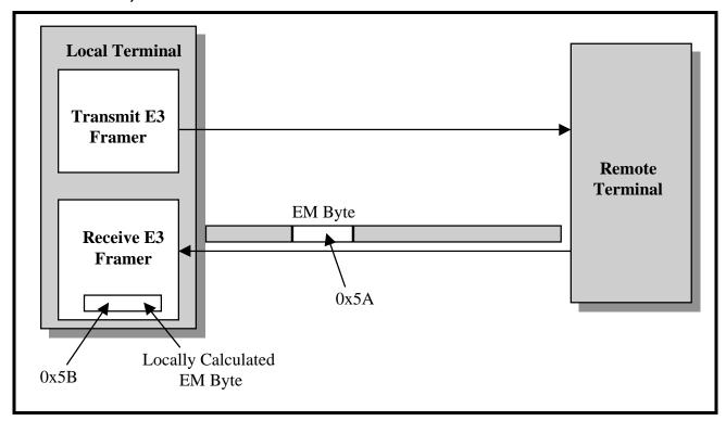
FIGURE 199. ILLUSTRATION OF THE LOCAL RECEIVE E3 FRAMER BLOCK, TRANSMITTING AN E3 FRAME (TO THE REMOTE TERMINAL) WITH THE FEBE BIT (WITHIN THE MA BYTE-FIELD) SET TO "1"
