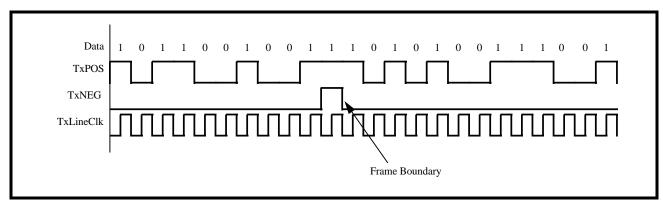
When the Transmit E3 LIU Interface block is operating in the Bipolar (or Dual Rail) mode, then the contents of the E3 Frame is output via both the TxPOS and Tx-NEG pins. If the Bipolar mode is chosen, then E3 data can be transmitted to the LIU via one of two differ-
