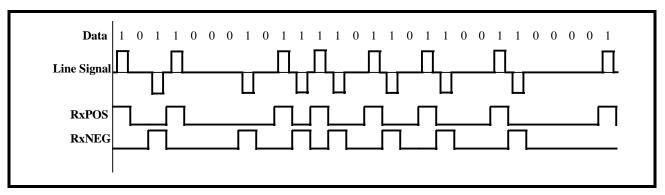
**Note:** One of the reasons that the AMI Line Code has been chosen for driving copper medium, isolated via transformers, is that this line code has no dc component, thereby eliminating dc distortion in the line.
