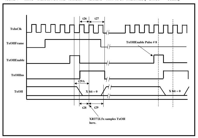
FIGURE 9. TRANSMIT LIU INTERFACE TIMING - FRAMER IS CONFIGURED TO UPDATE "TXPOS" AND "TXNEG" ON THE RISING EDGE OF "TXLINECLK"
