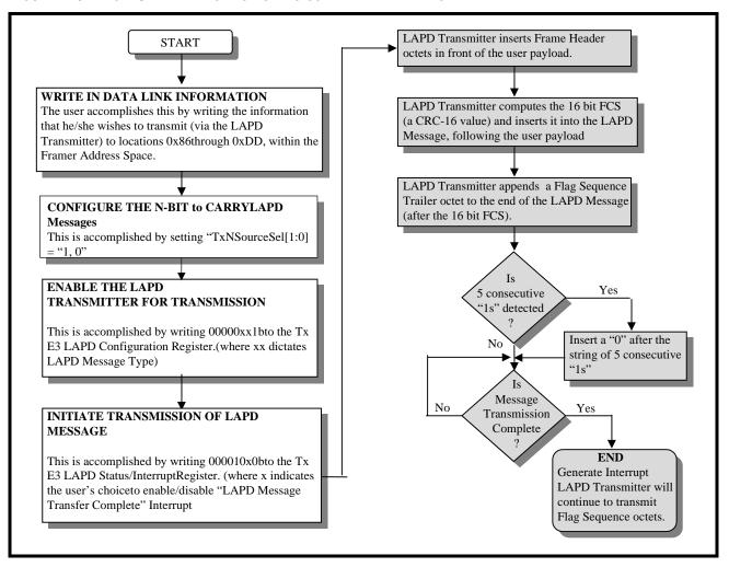
Note: In Figure 118, the unshaded boxes depict the tasks that the user must perform. The shaded boxes present the resulting tasks that the Transmit HDLC Controller block will perform.
