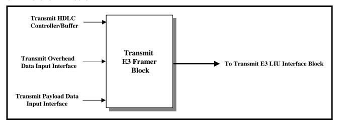
In addition to taking data from multiple sources and multiplexing them, in appropriate manner, to create the outbound E3 frames, the Transmit E3 Framer block has the following roles.
