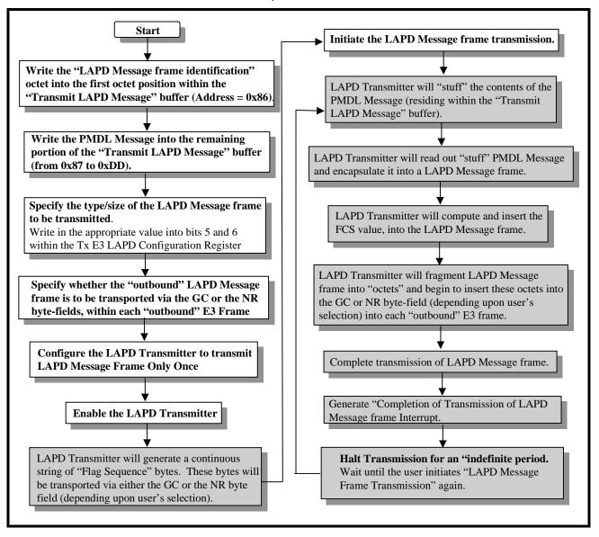
The Mechanics of Transmitting a New LAPD Message frame, if the LAPD Transmitter has been configured to re-transmit the LAPD Message frame, repeatedly, at One-Second intervals.
