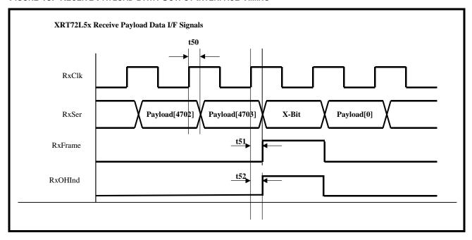
FIGURE 14. RECEIVE PAYLOAD DATA OUTPUT INTERFACE TIMING (NIBBLE MODE OPERATION)
