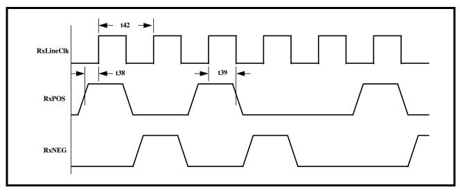
FIGURE 134. WAVEFORM/TIMING RELATIONSHIP BETWEEN RXLINECLK, RXPOS AND RXNEG - WHEN RXPOS AND RXNEG ARE TO BE SAMPLED ON THE FALLING EDGE OF RXLINECLK
