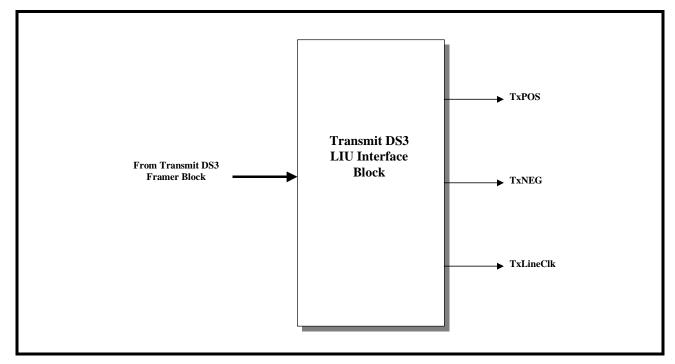
The Transmit DS3 LIU Interface block can transmit data to the LIU IC or other external circuitry via two different output modes: Unipolar or Bipolar. If the Unipolar (or Single Rail) mode is selected, then the contents of the DS3 Frame is output, in a binary (NRZ manner) data stream via the TxPOS pin to the LIU IC. The TxNEG pin will only be used to denote the frame boundaries. TxNEG will pulse "High" for one bit peri-
