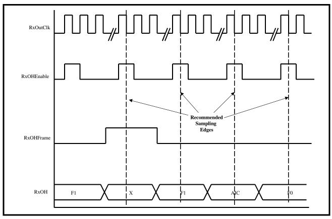
4.3.5 The Receive Payload Data Output Interface
