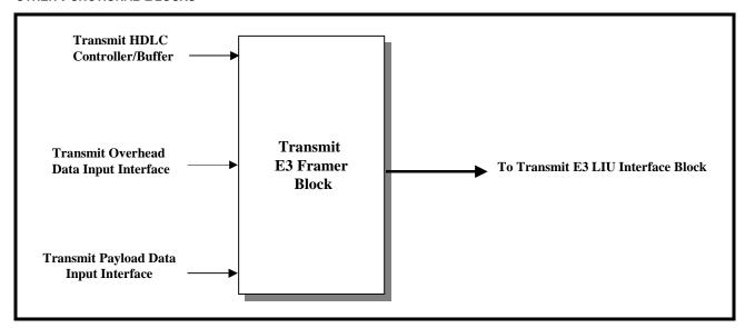
In addition to taking data from multiple sources and multiplexing them, in appropriate manner, to create the Outbound E3 frames, the Transmit E3 Framer block has the following roles.
