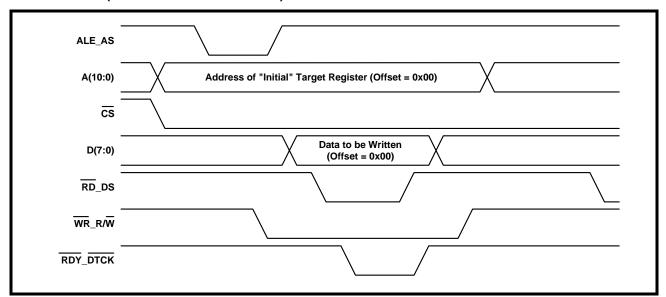
At the completion of this initial write cycle, the  $\mu$ C/ $\mu$ P has written a byte or word into the first register or buffer location (within the XRT72L54 DS3/E3 Framer) for this particular burst I/O access. In order to illustrate how this burst I/O cycle works, the byte (or word) of data, that is being written in Figure 35 has been labeled Data to be Written (Offset = 0x00).
