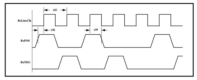
FIGURE 79. WAVEFORM/TIMING RELATIONSHIP BETWEEN RXLINECLK, RXPOS AND RXNEG - WHEN RXPOS AND RXNEG ARE TO BE SAMPLED ON THE FALLING EDGE OF RXLINECLK
