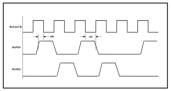
FIGURE 12. RECEIVER LIU INTERFACE TIMING - FRAMER IS CONFIGURED TO SAMPLE "RXPOS" AND "RXNEG" ON THE FALLING EDGE OF "RXLINECLK"
