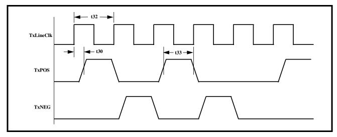
FIGURE 71. WAVEFORM/TIMING RELATIONSHIP BETWEEN TXLINECLK, TXPOS AND TXNEG - TXPOS AND TXNEG ARE CONFIGURED TO BE UPDATED ON THE FALLING EDGE OF TXLINECLK
