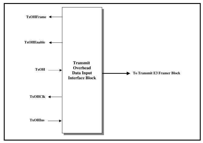
The E3, ITU-T G.832 Frame consists of 537 bytes. Of these bytes, 530 bytes are payload bytes and the remaining 7 are overhead bytes. The XRT72L54 has been designed to handle and process both the payload type and overhead type bits for each E3 frame. Within the Transmit Section within the XRT72L54, the Transmit Payload Data Input Interface has been designed to handle the payload data. Likewise, the Transmit Overhead Input Interface has been designed to handle and process the overhead bits.
