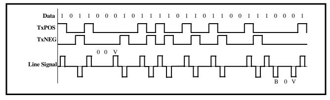
The user chooses between AMI or B3ZS line coding by writing to bit 4 of the I/O Control Register (Address = 0x01), as shown below.
