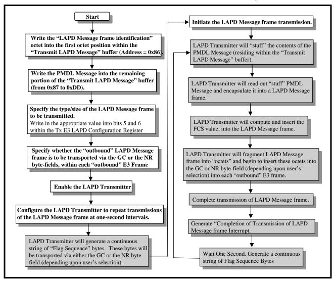
Figure 176 presents the procedure (in white boxes) which the user should use in order to transmit a PM-DL Message via the LAPD Transmitter, when the
