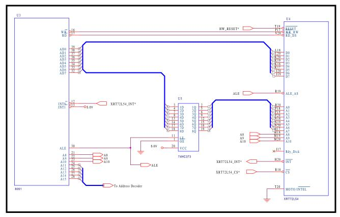
The circuitry in Figure 37 will function as follows, during a Framer-request interrupt. The Framer device would request an interrupt from the CPU by asserting its active low  $\overline{\text{INT}}$  output pin. This will cause the INT0\* input pin of the CPU to go "Low". When this
