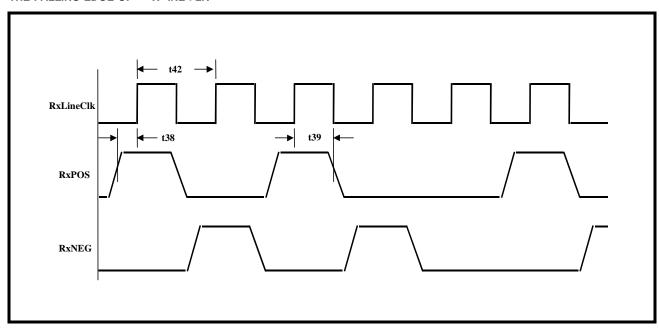
FIGURE 13. RECEIVE PAYLOAD DATA OUTPUT INTERFACE TIMING
