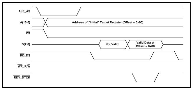
At the completion of this initial read cycle, the  $\mu C/\mu P$  has read in the contents of the first register or buffer location (within the XRT72L54 DS3/E3 Framer) for this particular burst access operation. In order to illustrate how this burst I/O cycle works, the byte (or word) of data, that is being read in Figure 33 has been labeled Valid Data at Offset = 0x00. This indicates that the  $\mu C/\mu P$  is reading the very first register (or buffer location) in this burst access.
