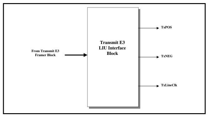
The Transmit E3 LIU Interface block can transmit data to the LIU IC or other external circuitry via two different output modes: Unipolar or Bipolar. If the user selects Unipolar (or Single Rail) mode, then the contents of the E3 Frame is output, in a binary (NRZ manner) data stream via the TxPOS pin to the LIU IC. The TxNEG pin will only be used to denote the frame boundaries. TxNEG will pulse "High" for one bit peri-
