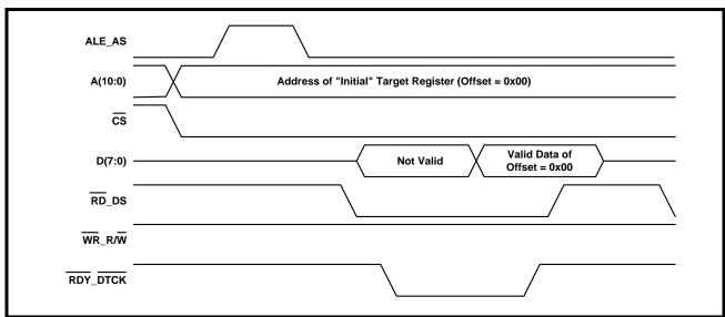
At the completion of this initial read cycle, the  $\mu C/\mu P$  has read in the contents of the first register or buffer
