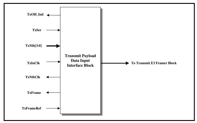
Each of the input and output pins of the Transmit Payload Data Input Interface are listed in Table 71 and described below. The exact role that each of these
