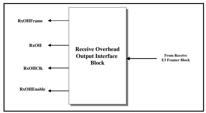
The E3, ITU-T G.751 frame consists of 1536 bits. Of these bytes, 1524 bits are payload bits and the remaining 12 bits are overhead bits. The XRT72L54 has been designed to handle and process both the payload type and overhead type bits for each E3 frame.
