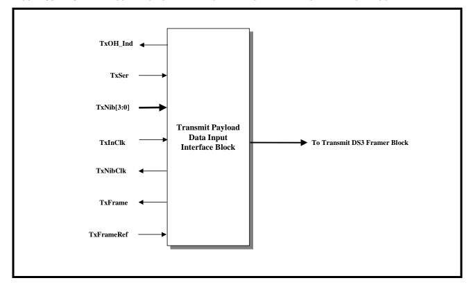
Each of the input and output pins of the Transmit Payload Data Input Interface are listed in Table 47 and described below. The exact role that each of these
