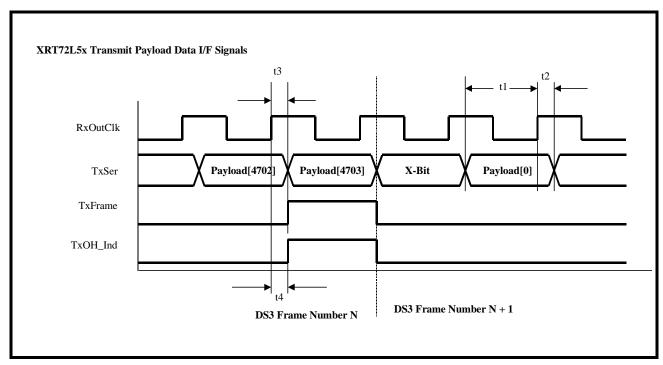
FIGURE 4. TIMING DIAGRAM FOR THE TRANSMIT PAYLOAD INPUT INTERFACE, WHEN THE XRT72L54 DEVICE IS OPERATING IN BOTH THE DS3 AND LOCAL-TIMING MODES
