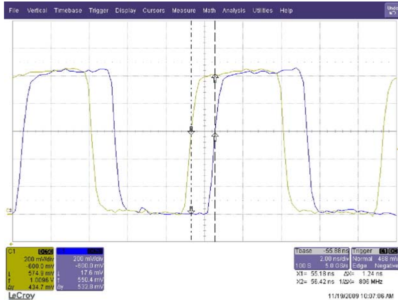
Figure 12. Scope Plot - Phase Skew Adjustment
