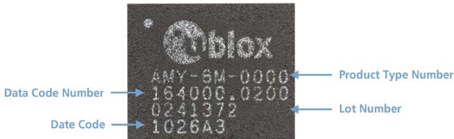
Figure 7: Location of product type number on AMY-6M packages
