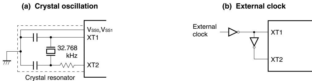
Figure 5-6. External Circuit of Subsystem Clock Oscillator
