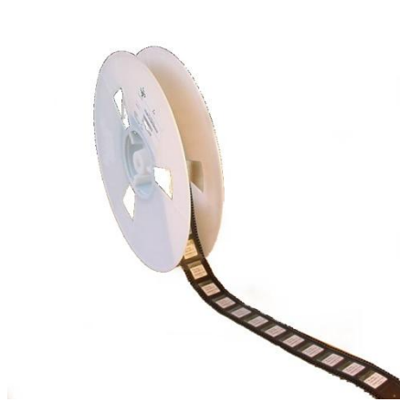
Figure 4: Reeled u-blox modules
