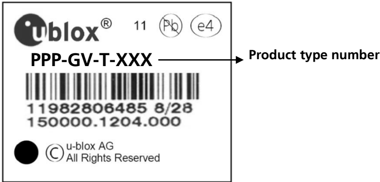
Figure 7: Location of product type number on u-blox 6 module label
