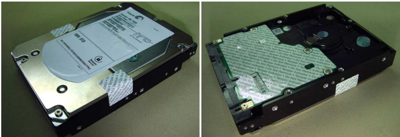
Figure 8. Example of FIPS tamper evidence labels.
