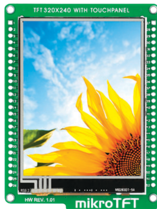
Figure 2: mikroTFT display board
