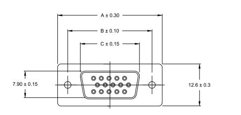
ELECTRICAL: INSULATOR RESISTANCE: WORKING VOLTAGE: OPERATING TEMPERATURE: CONTACT RESISTANCE: CONTACT AMPERAGE: MATERIALS: CONTACTS:
