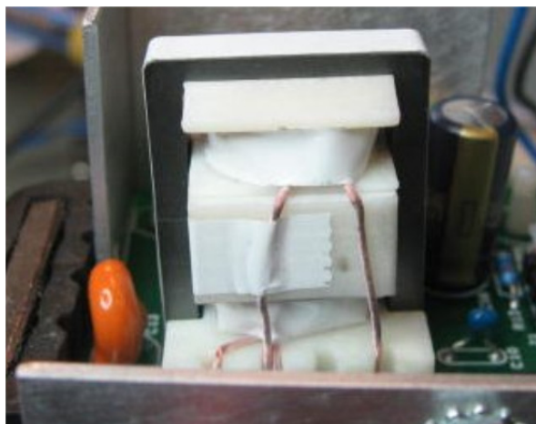
Figure 49 – Visible Light Transformer Front View.
