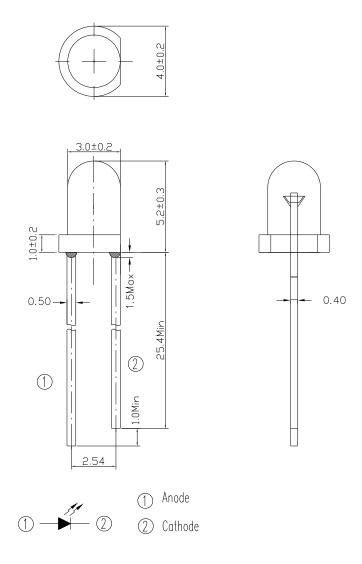
Note: Tolerances unless dimensions ±0.25mm
