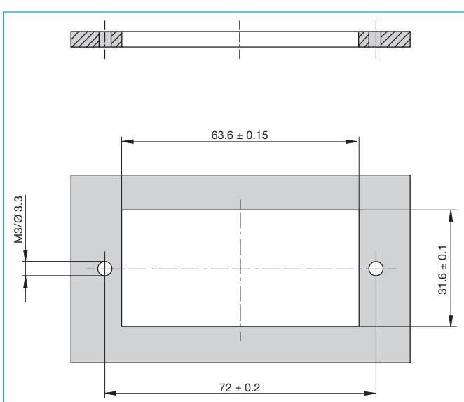
This is a metric design and millimeter dimensions take precedence ( $\frac{\text{mm}}{\text{inch}}$ )
