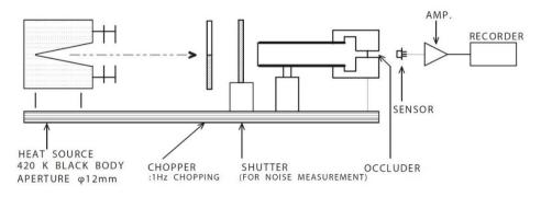
Figure 2 - Occluder Position
