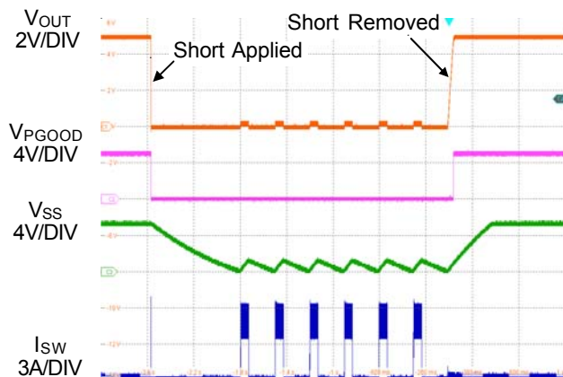
Figure 3. Short-Circuit Protection and Recovery
