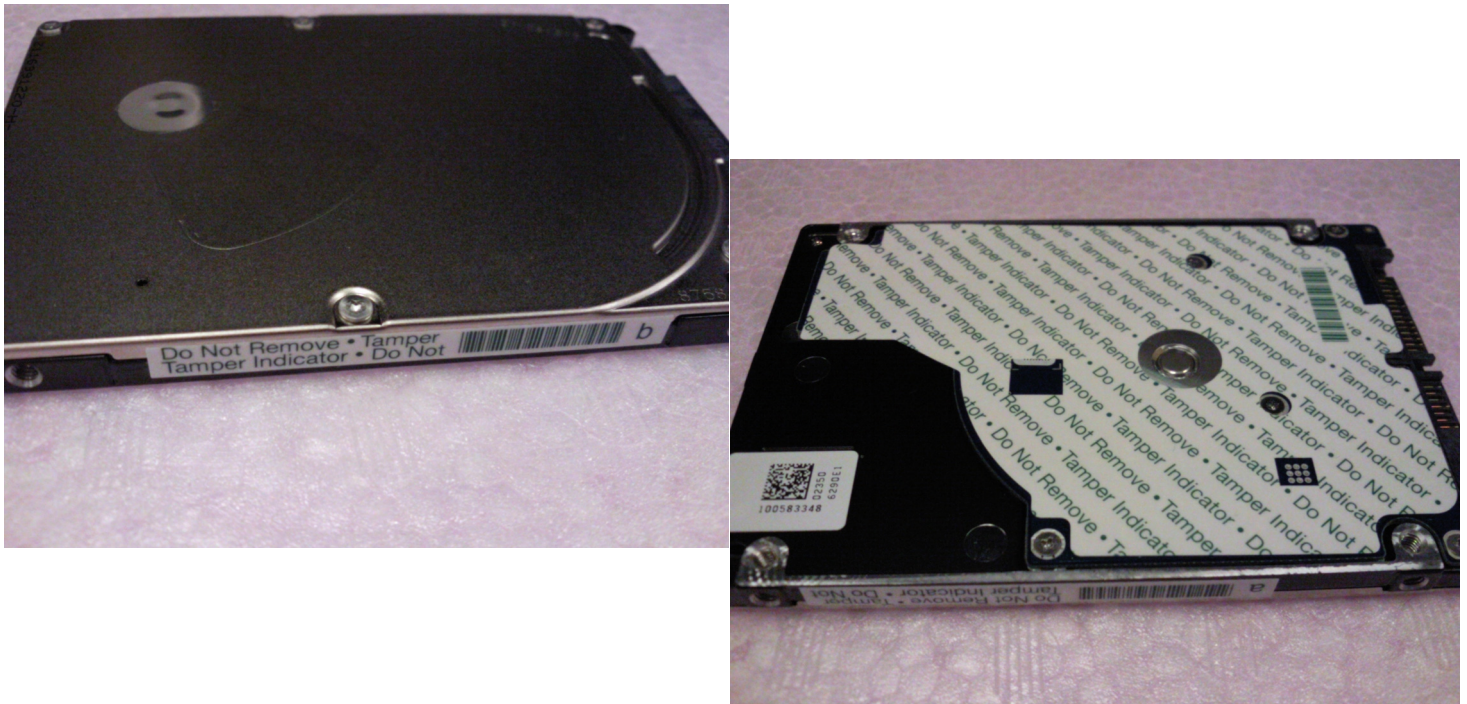
Figure 6 Example of FIPS tamper evidence labels.
