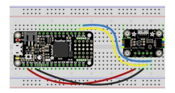
Board 3V to sensor VIN (red wire on STEMMA QT version) Board GND to sensor GND (black wire on STEMMA QT version) Board SCL to sensor SCL (yellow wire on STEMMA QT version) Board SDA to sensor SDA (blue wire on STEMMA QT version)
