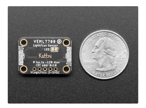
Interfacing is easy - this sensor uses plain, universal I2C. We put this sensor on a breakout board with a 3.3V regulator and logic level shifter so you can use it with 3.3V or 5V power/logic microcontrollers. We have written libraries for Arduino (https://adafru.it/EoE) (C/C++) as well as CircuitPython (Python 3) (https://adafru.it/EoF) so you can use this sensor with just about any kind of device, even a Raspberry Pi!
