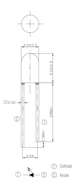
Note: Tolerances unless dimensions ±0.25mm
