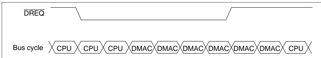
Figure 11.13 DMA Transfer Example in the Burst Mode
