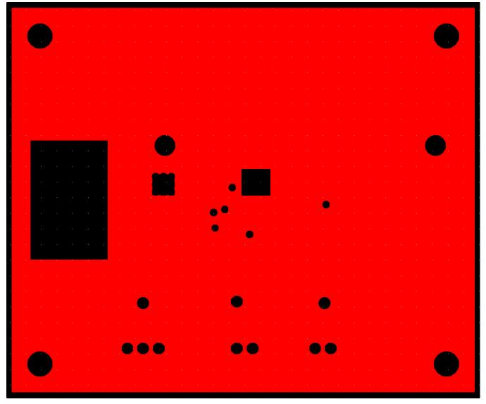
Figure 5-3. GND Plane (Layer 2)
