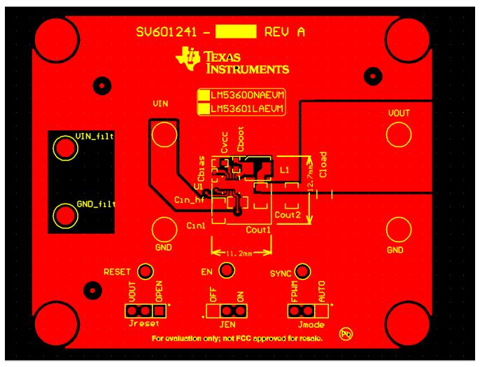
Figure 5-1. Top Layer with Overlay
