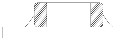
Not enough solder Weak holding force may cause bad connections or detaching of the capacitor
