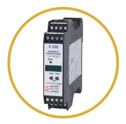
The SC-E-100 Ethernet Gateway module provides a straight forward method of interfacing analogue and digital process parameters to an Ethernet or RS232/485 network. The SC-E-100 allows the user to view the status of the individual inputs via the front panel display.
