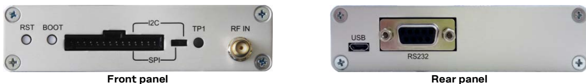
Figure 2: EVK-M8T evaluation unit – front and rear panels
