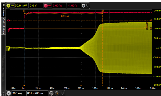
Figure 24. Switching Time [Isolation to Insertion Loss State]
