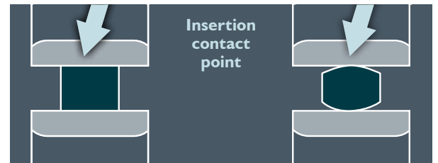
Figure 3: To assume that the use of normal force predicts contact performance is flawed thinking. The domed connector on the right delivers greater reliability because the normal forces are being channeled through a smaller area. Thus, there is more force per unit area available to penetrate the one obstacle standing in the way of stable contact resistance: contact films. (Image: Can Your Connectors Pass the Ultimate Stress Test?)
