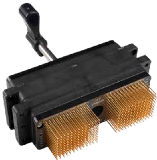
Figure 2: This 156-pin connector is part of the Cannon DL series of ZIF connectors. The cam in the center is the basis for zero force insertion. Single-handed actuation makes it easy to mate. A broad range of pin count, size, materials, and performance options are available for finding the exact choice. (Image: ITT Cannon)
