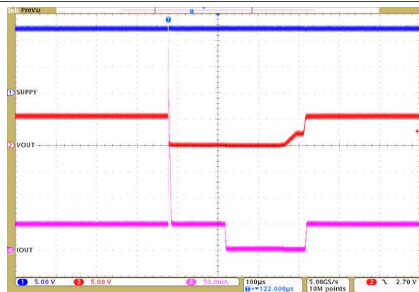
Figure 11. LED Short-Circuit Protection and Recovery
