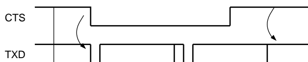
Figure 20-16. Transmitter Behavior when Operating with Hardware Handshaking
