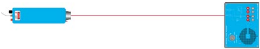
Figure 8. Class IIIa laser and laser beam aligned with an Industrial Fiber Optics' audio laser receiver for demodulation of the laser beam's modulated signal and producing sound waves.
