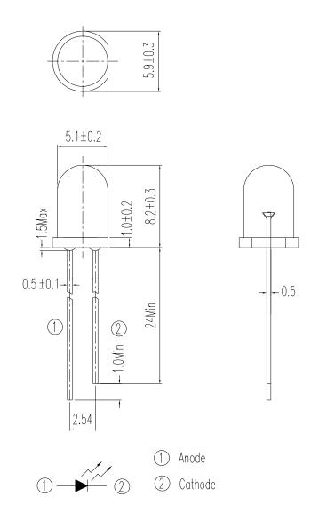
Note: Tolerances unless dimensions ±0.25mm
