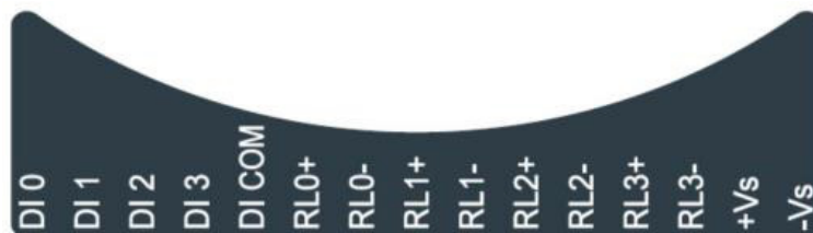
Figure 2.34 WISE-4060 Pin Assignment
