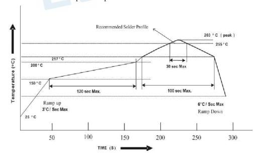
3.2 Reflow soldering should not be done more than two times.
