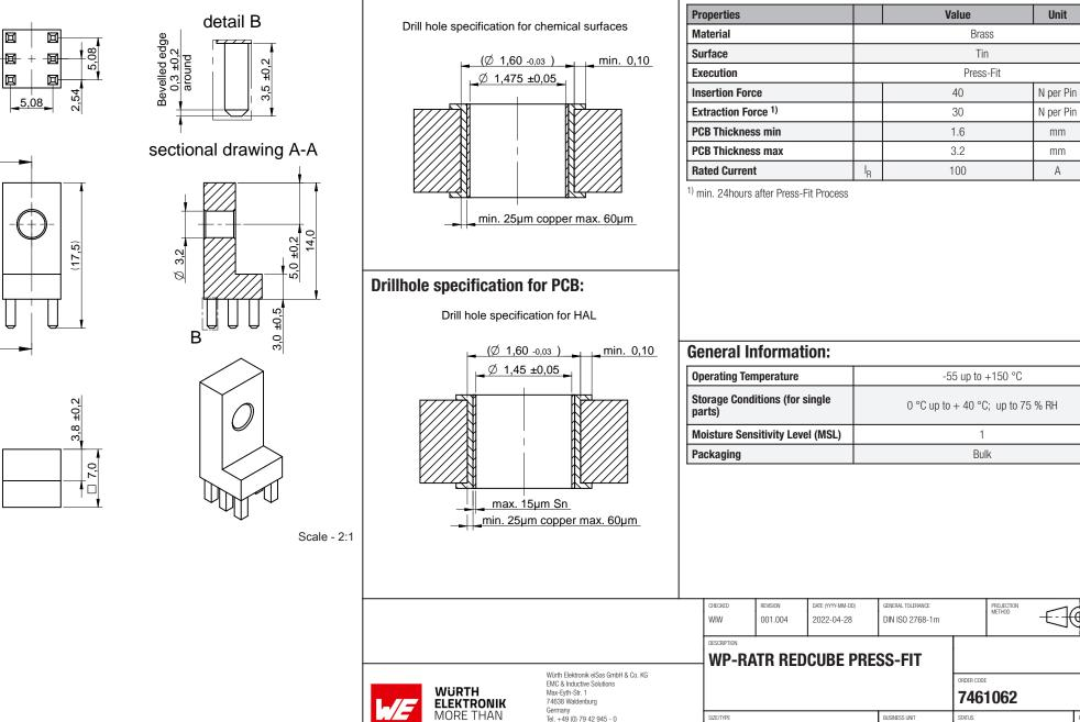
**Drillhole specification for PCB:**
