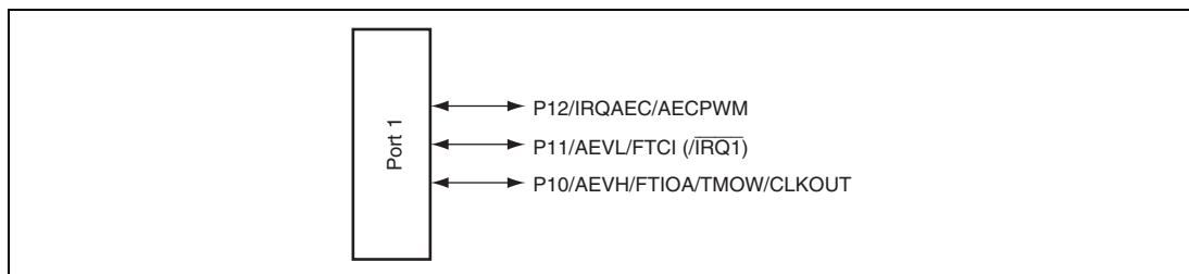
Figure 8.1 Port 1 Pin Configuration
